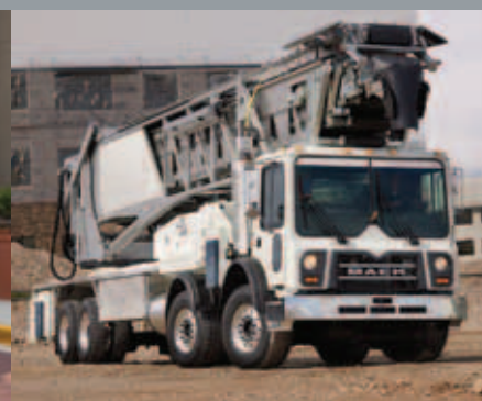
CONCRETE CONVEYOR BELT
